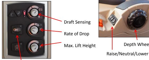
Active Transport (3-point hitch suspension system)
