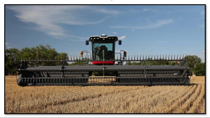
5300 Series headers allow producers to utilize the WR9800 Series windrower in a grain swathing application.
