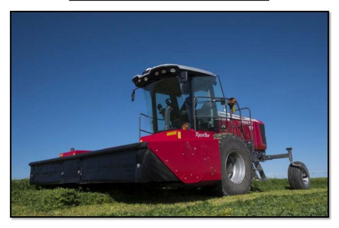
Producers may equip their WR9860 or WR9870 Series windrower with one of 4 9100 Series disc headers. These headers are available in 13' or 16' configurations and fitted with single steel on steel conditioners, or Twin Max dual steel on steel conditioners.
