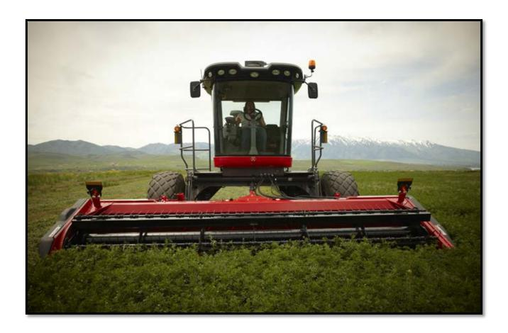
Producers may equip their WR9800 Series windrowers with a sickle auger header if needed. These headers are available in 14', 16' or 18' configurations.
