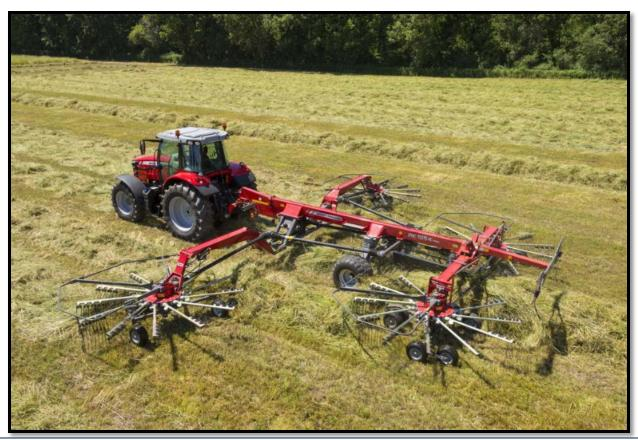
Operations looking to produce top quality hay or forage would be best served with one of our 8 rotary rake models in the RK Series lineup. By their design, RK Series rotary rakes ensure windrows are built free from excess ash or debris, and with a light, fluffy consistency that improves crop dry down as well as baler feeding.
