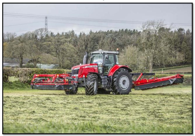
The DM Series lineup includes the DM306 front mower, and DM9314 rear butterfly mowers. This triple mower setup allows larger scale operations to mow 30' 6" in a single pass.
