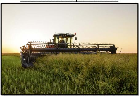
The introduction of the 5400 Series draper header allows any of the 4 WR9900 Series windrowers to be utilized in a grain swathing application. 5400 Series headers are offered in 5' increments from 20'-40' with center delivery or double swath configurations. They also include multiple developments to ensure we have an industry leading draper head paired to the industry's best windrower tractor.
