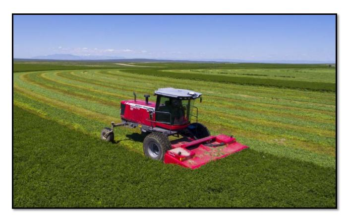
The WR9800 Series includes 3 models of windrowers capable of performing multiple tasks, from swathing grain to moving and conditioning different crops with disc or sickle headers.
